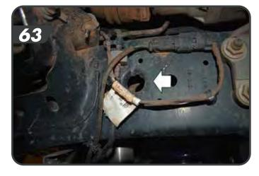
g. Insert the Long single nut tab [64, 65)] into the frame from the outside large frame hole. Use the provided ½" hardware hold it in place. Leave loose.
