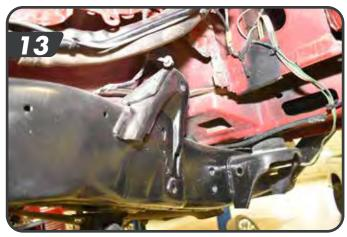
Grind the formed support rib at a taper. Starting at  $3-\frac{3}{4}$ " down from the top of the shock mount to the bottom of the rib being flushed with the frame. [14]
