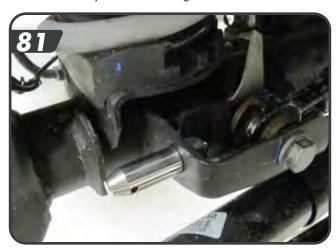
h. Install the longer disconnect post on the driver side axle sway bar link mount with it pointing inboard [82]. Fasten with the ½" nylock nut and tighten to 64 ft-lbs. Tighten the post with the pin hole parallel to the ground. Slide the polyurethane spacer on the pin up against the axle tab.
