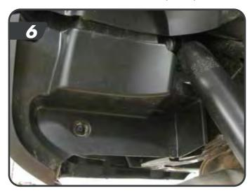
Remove the rest of the inner fender liner by removing six factory plastic rivets and the plastic body clips [7].
