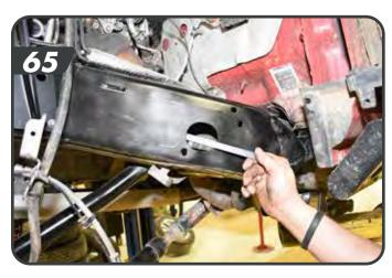
h. One at a time remove each ½" bolt and use the provided loctite. Torque the steering box bolts (18mm) to 99 ft-lbs and the ½" hardware (¾" to 90 ft-lbs. Leave the brake line bracket bolt loose.
