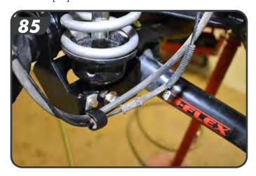
m. Reattache the factory brake line to the frame through the frame mount with OE hardware (10mm). Torque Bolt to 115 in-lbs.
