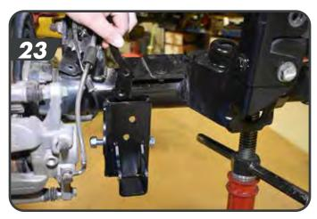
c. Insert the nut tab [24] on the front side of the lca pocket and use the provided 7/16" bolts and washers to mount the axle mount through the holes you opened up previously to ½". [25] Torque the 7/16" bolt (5/8") to 59 ft-lbs.
