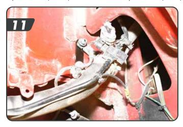
a. Using a cut off wheel and reciprocating saw (plasma cutter can be used too) cut off the outter shock tab flush with the inner shock mounting surface. [12, 13] Grind surface smooth with Shock mounting surface.
