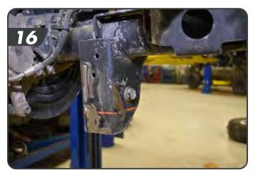
i. Using a cut off wheel or reciprocating saw remove 1-34" from the bottom of the LCA mount measured from the rear bottom keeping the cut horizontal. [17, 18]
