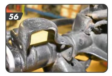
d. using a small (3") cut off wheel or Recipricating saw cut the shock mount off of the axle as close to the axle as possilbe without hitting the axle. [57]
