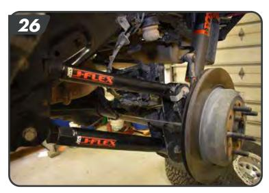
g. Mount the control arm to the frame bracket with the grease fitting up. Install the original mounting bolt and flag nut. Finger tighten the bolt. [27] DO NOT torque mounting hardware until instructed.
