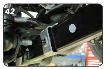
Disconnect the brake line from the axle coil mount location [43] Remove the axle braket and LCA braket from the brake line.
