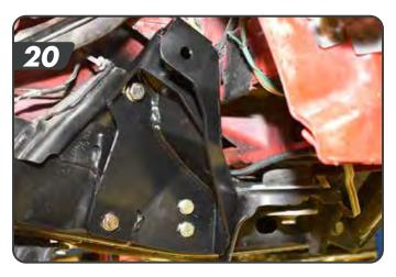
b. Mark the rear facing hole on the body mount and remove the bracket. Drill the hole to ½". Paint any Bare surfaces. [21]
