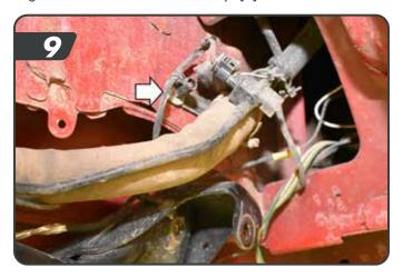
c. Loosen the forward filler neck mount and and lift filler neck and retighten hardware. [10]
