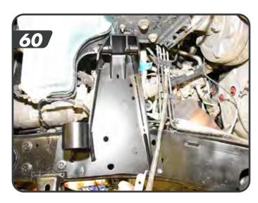
c. Remove the forward factory fastener holding the heat sheild to the motor mount bracket. Mount the Frame Coilover Reinforcement Bracket to the factory motor mount bracket with the provided 3/8" bolt, nut and washer in bolt pack J137. Leave hardware loose[61]
