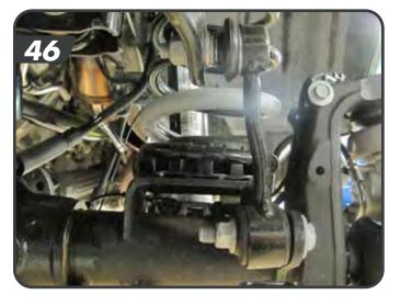
i. Remove the 4 bolts mounting the front driveshaft to the pinion flange (15mm) and support it with a strap or bungee cord. This is done to ensure the driveshaft does not bind when removing the coil springs. [47]
