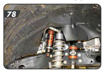
b. Fasten the inner fenders to the body with the original hardware. Use the provided Plastic rivets and a standard Rivet gun mount the inner fender to the fender.
