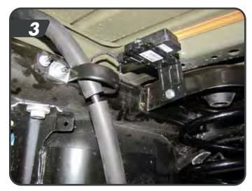
Rubicon models: Disconnect the locker wires from the differential.
