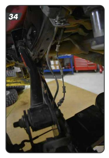
g. Reatcch the brake line to the axle mount with OE hardware (10mm). Also use the provided cable tie and attach the brake line to the abs wire. [35]
