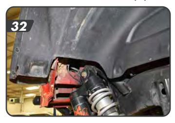
b. Fasten the inner fenders to the body with the original hardware/clips and new plastic rivets.
