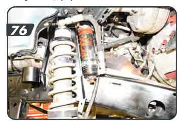
c. Raise the axle to mount the coilover into the lower mount. Fasten with the ½" x 2-¾" bolt washer and nut. [77]
