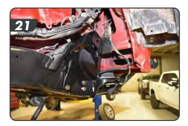
c. Remount the frame mount as before. Use the provided 7/16" bolt, washer, and nut through the body mount hole just drilled. Torque all hardware to the following. [22] 12mm (19) 81ft-lbs, 10mm (17) 45 ft-lbs, 7/16" (5/8") 59 ft-lbs.
