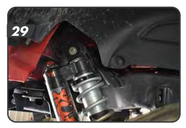
b. Raise the axle to mount the coilover into the lower mount. Fasten with the ½" x 2-¾" bolt, washers, and nut. [30, 31]
