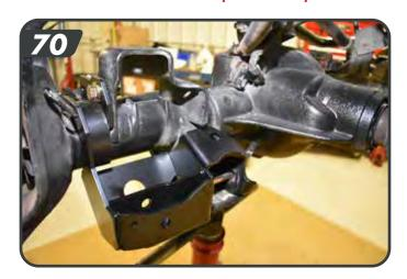
q. Mark the location of the most forward holes location on the coil mount. Remove the bracket and drill with a 7/16" Bit. Paint any raw metal.
