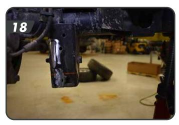
j. Drill out both holes in the rear of the lca bracket to ½" [19].
