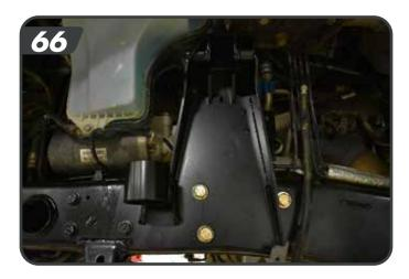
i. Mount the Frame Coilover Reinforcement Bracket to the Frame Mount Bracket with the Remote Resi Bracket using the provided 5/16" (½" socket and wrench) bolts, nuts, and Washers. [67] Torque hardware to 178 in-lbs
