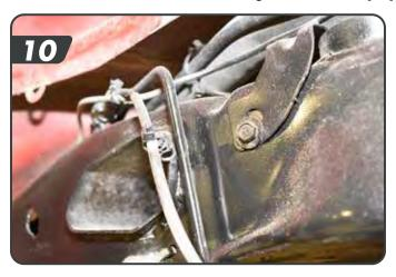
d. Install the Fuel filler neck relocation bracket to raise the neck up away from the shock mount. [11] Using the ¼" washer and nut in bolt pack J145. Torque OE bolt (10mm) to 53in-lbs and torque ¼" nut (7/16) to 86 in-lbs.
