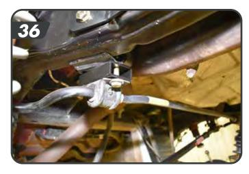
Set the length of the provided rear sway bar links with the booted joints to 11-1/4" between the ball stud centers and install to the outside of the sway bar and axle mount [37a, 37b]. Torque to 72 ft-lbs.
