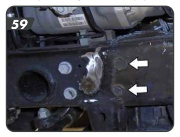
b. Adjust the hard brake lines out of the way. Place the Frame Mount Bracket onto the frame lining up the two front holes and the brake line bracket hole. Mark the center of the remainder of the holes. Remove the bracket from the frame and drill all the holes to 9/16". [60] Paint all raw metal.
