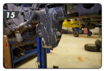
h. Use a cut off wheel or reciprocating saw Remove the Axle sway bar mount from the LCA mount. grind the LCA mount smooth. [16]
