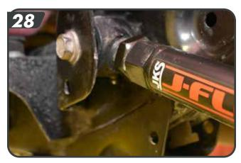
**HINT:** If mounting bolt is difficult to install due to misalignment of Control Arm bushing with mounting bracket, either (1) adjust height of axle housing with hydraulic jack, or (2) move axle housing into position with a heavy-duty ratchet strap.
