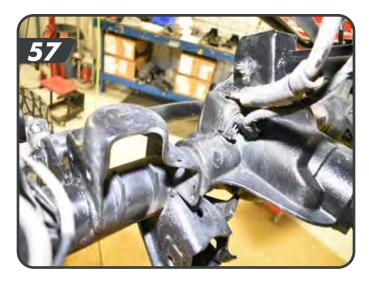
e. Using a cut off wheel cut the LCA mount flange of the axle as shown. [58]
